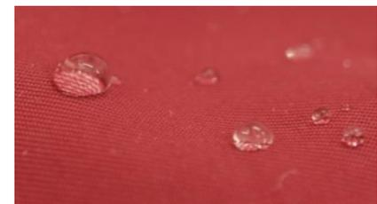
The full impregnation of the fiber using our specially developed fixing-technique ensures long-term protection (in contrast to the processes of conventional laundry services)
